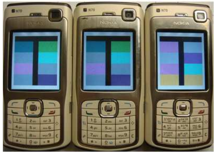
Fig. 4. Our Mobile Client displaying T-Flags on N70 smart phones during a SPATE exchange. The left and center T-Flags are identical, but the right T-Flag is different.
