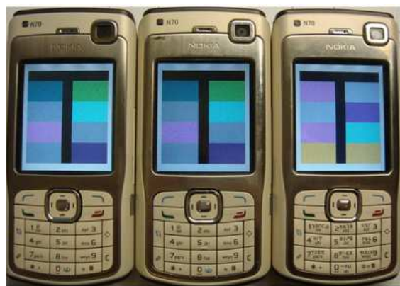
Figure 4: Our Mobile Client displaying T-Flags on N70 smart phones during a SPATE exchange. The left and center T-Flags are identical, but the right T-Flag is different.
